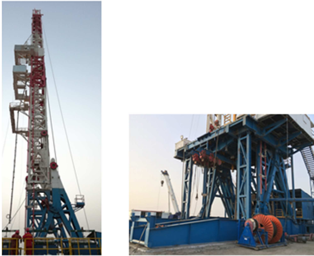
Figure 1. Derrick and Substructure of Quadruple Joint Drilling Rig.
