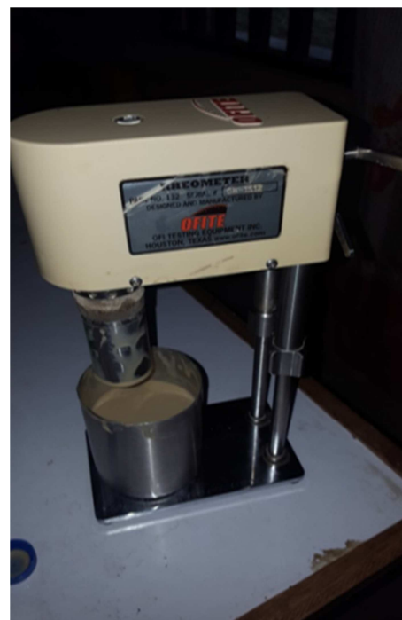
Figure 5. Viscometer with a prepared mud sample for rheology test.
