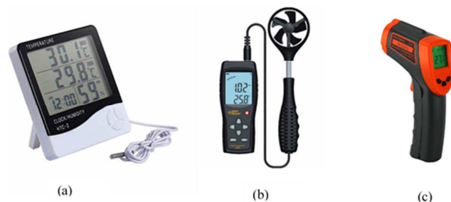
Figure 3. Field survey measurement tools (a) hygrometer, (b) anemometer and (c) infrared thermometer.
