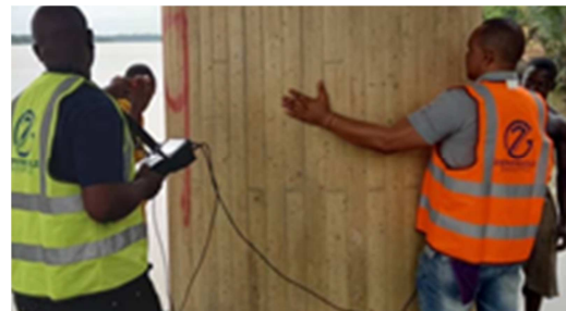
Figure 3. Testing of Piers using UPV.
