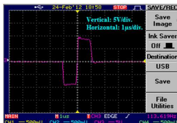
Figure 4. Output signal shape of DLA.
