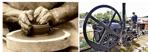
Figure 3. Potters wheel & Trevithick's 1802 steam locomotive using a flywheel to evenly distribute the power of its single cylinder to present [5].
