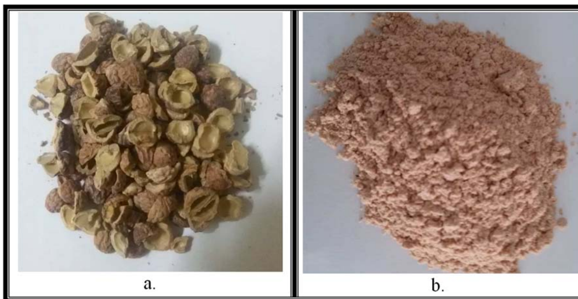
Figure 1. Shell's seeds of Ziziphus spina christi a. before grinding, and b. after grinding.
