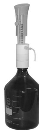
Figure 9. Dosing device for dosing barium chloride solution into selected doses of soil extract.
