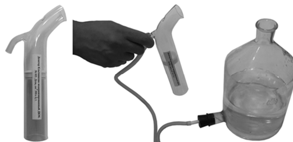
Figure 3. Klychnikov's one-position manual dispenser. On the left is a separate dispenser, on the right is an assembly.
