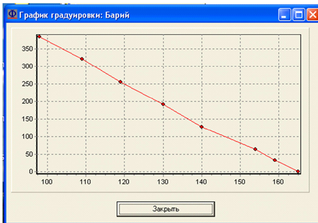
Figure 10. Calibration plot of the dependence of the quantitative content of barium (Y-axis) on the concentration of sulfates in solution (X-axis). Relative values.
