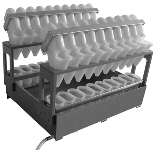
Figure 7. Filter unit BFM-2 for filtering soil suspension from KBM cassettes into KMM cassettes.
