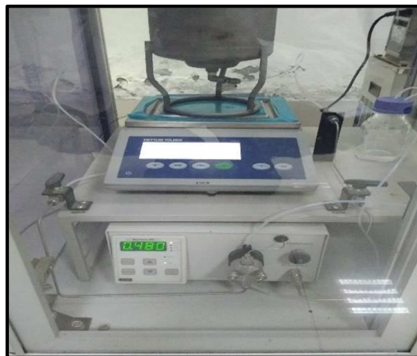
Figure 8. Liquid feed section.
