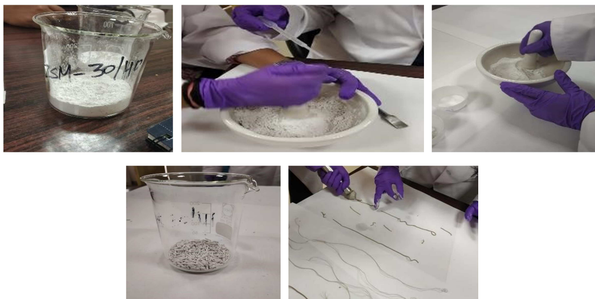
Figure 4. Synthesis of Extruded ZSM-5.
