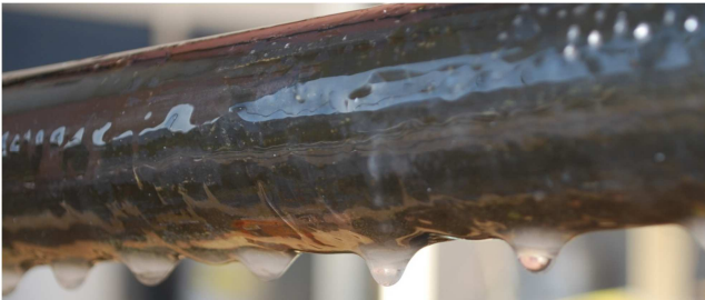
Figure 19. A glossy layer of ice surrounds the evaporator pipe with icicles forming underneath.
