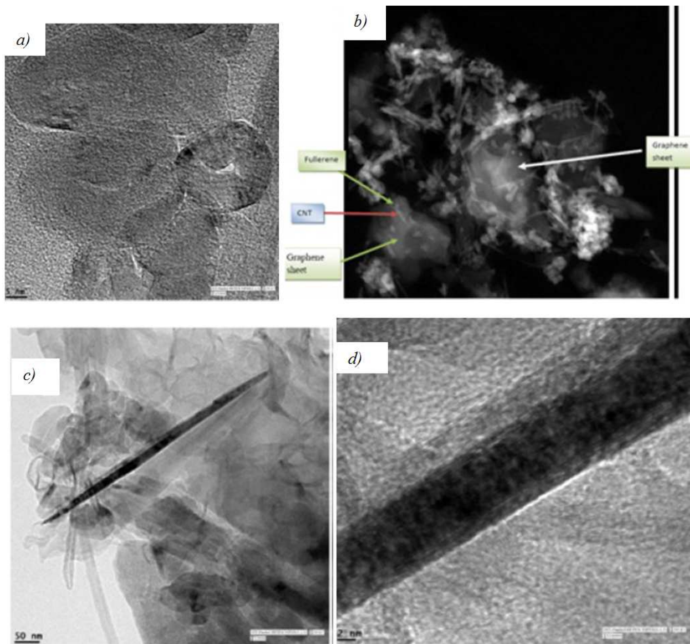
Fig. 5. HR-TEM and STEM images of CNTs prepared from Fe:C 1:1 molar ratio after purification a) HR-TEM images of high magnification of the nanorings/fullerene attached to each other b) STEM 3-D images of graphene sheet c) distribution of CNTs and fullerene on the surface of graphene sheet d) magnified form of panel c, showing morphology of CNT filled with iron particles.
