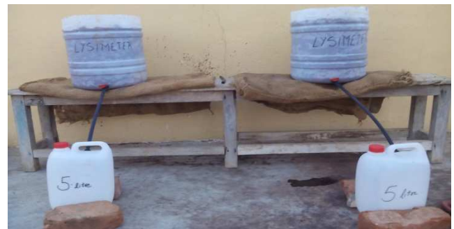
Figure 2. Lysimeter setup in the field.
