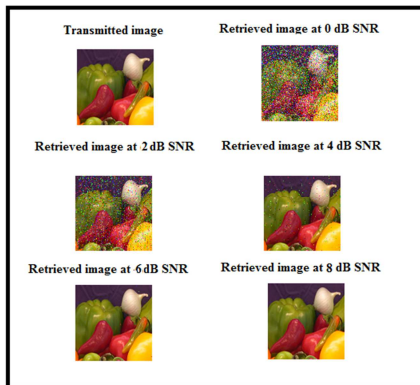
Figure 6. Transmitted and retrieved images in Hybrid Precoded Millimeter Wave Wireless Communication system under implementation of ZF signal detection, LDPC channel coding and 16-QAM digital modulation scheme.
