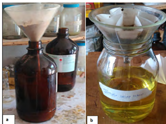
Figure 1. (a) Mixture of n Hexane and powered seed for extraction (b) Filtration of extracts.
