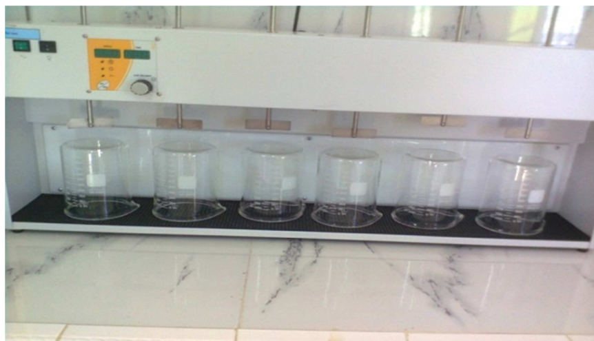
Figure 1. Jar test device used in coagulation test experiments.
