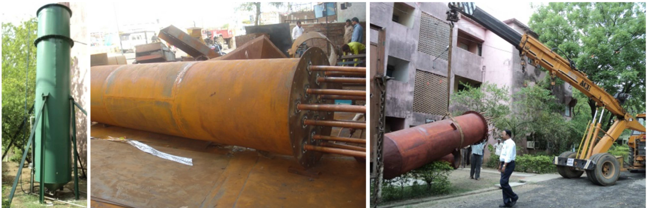
Figure 7. Fabrication of Heat Pipe Heat Exchanger.
