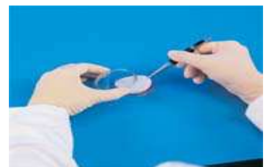
Fig. 5. Place the membrane filter into the prepared Petri dish.
