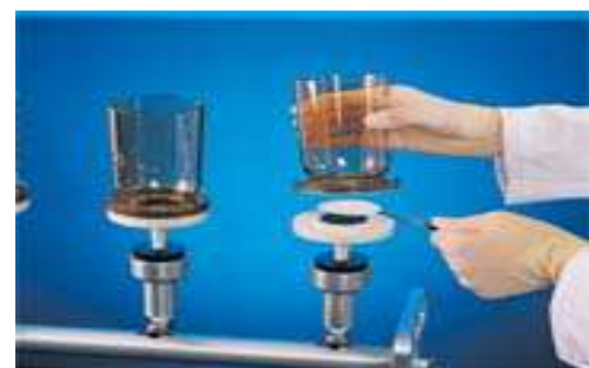
Fig. 4. Remove the membrane filter from the funnel.
