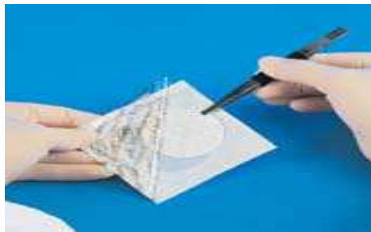
Fig. 2. Remove the membrane from the sterile package.
