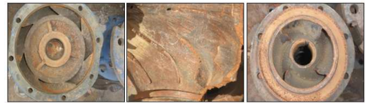
Figure 2. Pump housing immersed damaged by abrasion.
